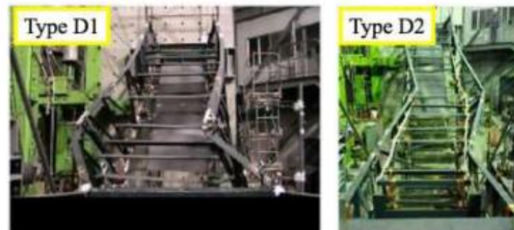
Figure 11 Deformation state of the type C1 and C2 escalator truss
