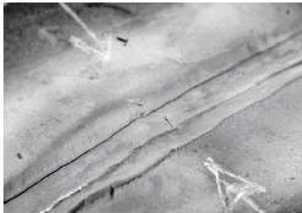
Cricca trasversale in zona fusa (Cricca a freddo – Controllo MT)
